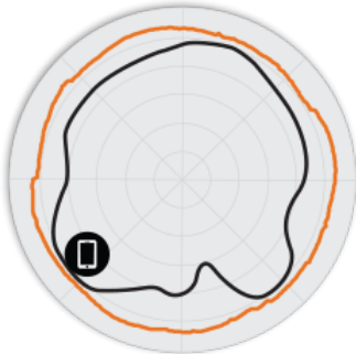
Figure 2. T310d 2.4GHz Azimuth Antenna Patterns
