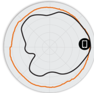
Figure 3. T310d 5GHz Azimuth Antenna Patterns
